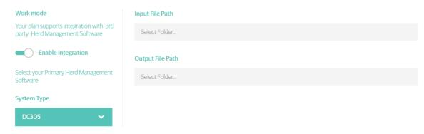
When choosing to work in DC305 or PC Dart Modes the input and output file paths must be defined. These are the file paths where DC305 / PC Dart places the Status File, Input File Path, and where SenseHub, Output File Path, places its output files.
